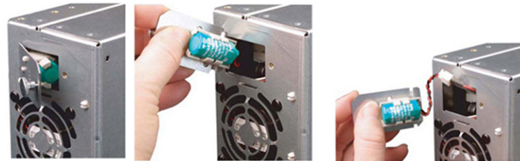
Example: PCU 50.3 battery replacement
