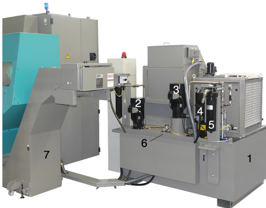
Example: Chip conveyor R200 with cooling lubricant cleaning system, immersion cooler and single filter
